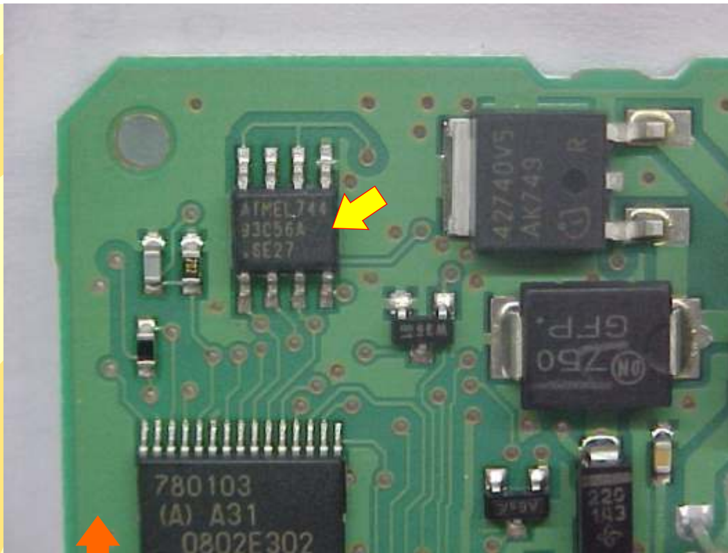
Conectando a Pinça Soic 8 na EEPROM serial 93C56
